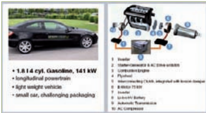
FIG. 6: ([4] DEIML, RAMPELTSHAMMER) PARALLEL HYBRID OF SIEMENS VDO
