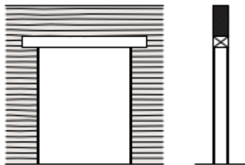
Figure 6: Lintel from another material 54
