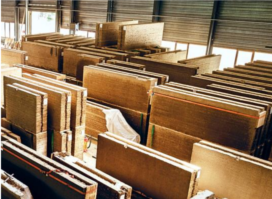
Figure 10: Drying of the rammed earth elements 78
