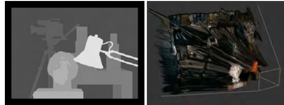
(c) Ground truth disparity map (left) and 3d rendering of the result with edge enhancement (right).
